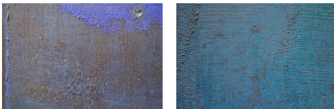
Figure 20:(left) thin layers of paint exhibit brittle appearance although are well adhered, figure 21: (right) directional brushstrokes originating from base layer. Photos taken by Eleanor Vallier.
